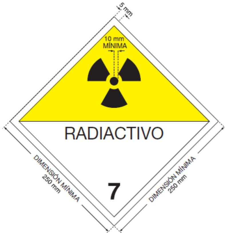
Figure A.6 Labeling. The dimensions of this model are the minimum; when using labels of different dimensions, the same proportions will be stored as in the model. The number "7" will have a
